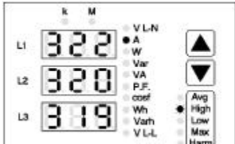
Esempio max corrente istantanea. Max instantaneous current example. L1=322A L2=320A L3=319A
